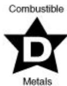
Extinguishers suitable for fires involving metals should be identified by a five-pointed star containing the letter 'D.' If colored, the star is colored yellow.\*
