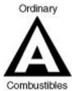
Extinguishers suitable for Class A fires should be identified by a triangle containing the letter 'A.' If colored, the triangle is colored green.\*
